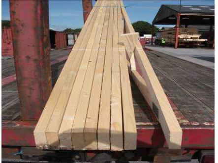
8. Once this wedge is in place the driver will then strap if possible the remaining bundle to the centre bars leaving the separated truss to be off loaded.
